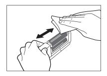
Load the Cleaning Roller and Cleaning Tape Cassette in order, and close the Front Cover.
