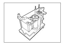
2 Push down the pin on top of the Transfer Film Cassette.
